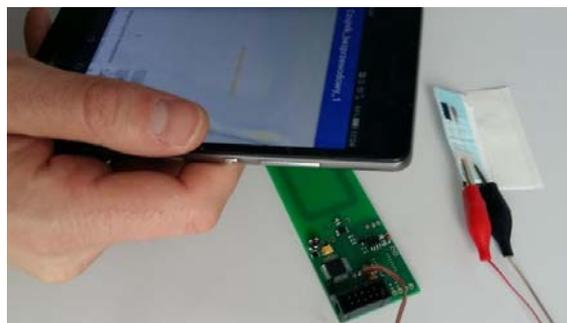
Fig. 2. NFC read-out device and sensor connected to the smartphone application for pH measurement.
