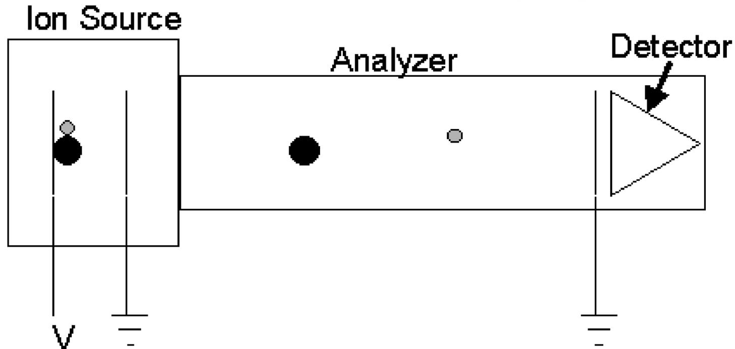
Mass spectrometer – ions are separated according to their mass-to-charge ratio in an analyzer
