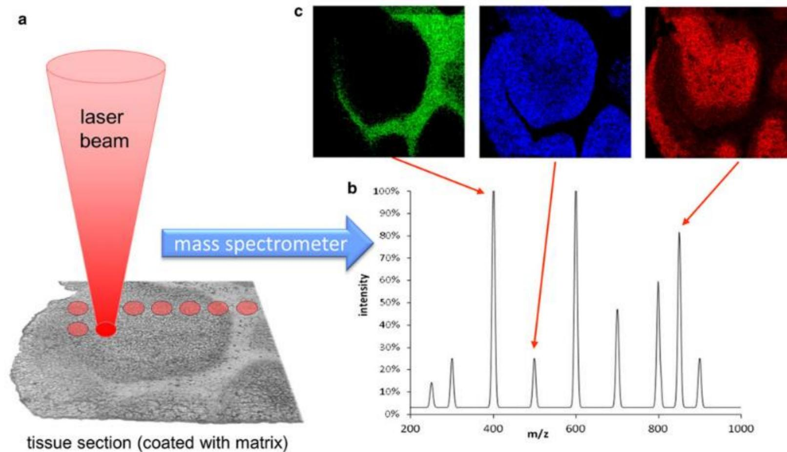
**Fig. 1** Scheme of the mass spectrometry imaging process. **a** The tissue section is covered with matrix and irradiated by a pulsed laser beam. **b** Mass spectrum acquired from the tissue section. **c** MS images of different  $m/z$  peaks
