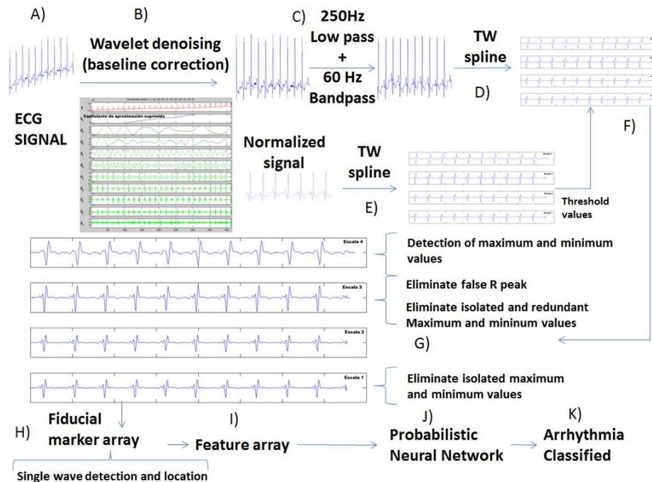
**Fig. 4.** Schematic diagram of the QWT/PNN arrhythmia classification process. A) The baseline of the original ECG signal B) is restored using a wavelet denoising process. C) The signal is filtered and D) transferred to the QWT section. E) A similar process is applied to the reference signal to obtain a set of threshold values. G) The QWT processed results in a set of H) fiducial markers and I) feature array. J) The PNN can then issue a result for K) arrhythmia classification.
