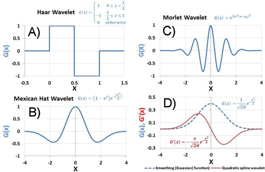
Fig. 2. Examples of reported wavelet functions used in ECG signal analysis. A) Haar, B) Mexican hat, C) Morlet and D) quadratic wavelets.
